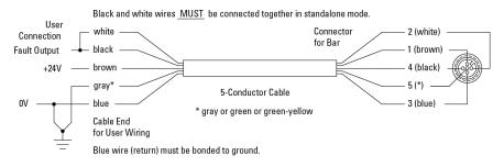
Figure 7: IQ Easy Static Bar Standalone Wiring
