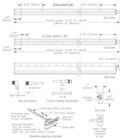
Figure 2: IQ Easy Static Bar Dimensions
