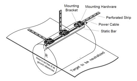
Figure 4: IQ Easy Static Bar Positioning
