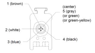
Figure 8: IQ Easy Static Bar Connector Pin-Out
